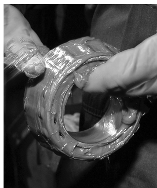
Fig. 15. Grease can easily be packed by hand.
